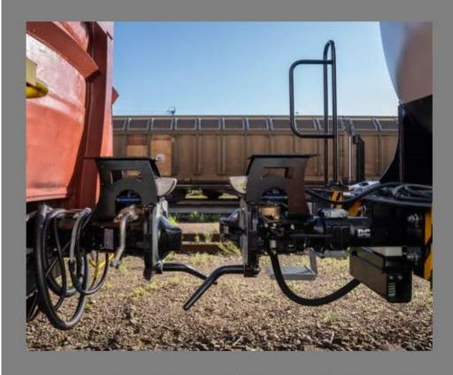
mechanical, pneumatical, energy & data coupling
